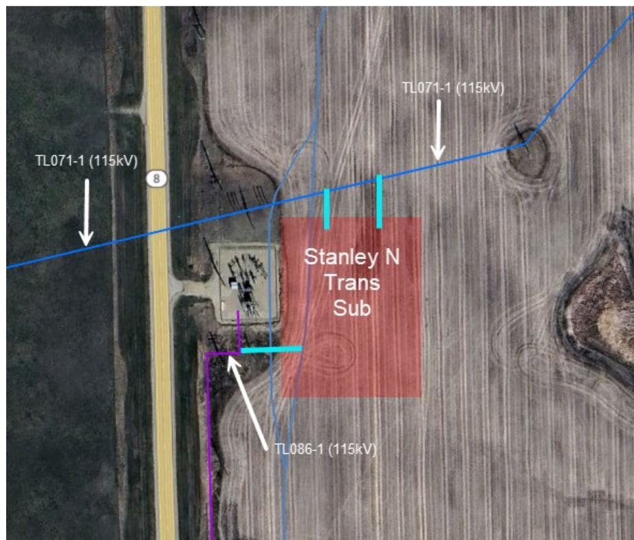
Transmission Line Reroutes
