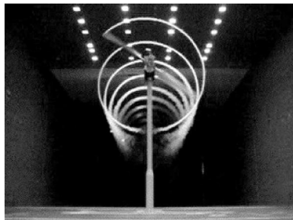
Fig. 7. Flow visualisation with smoke grenade in tip, revealing smoke trails for the NREL turbine in the NASA-Ames wind tunnel (from Hand [13]).
