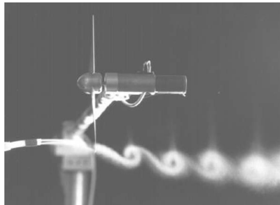
Fig. 6. Flow visualisation experiment at TUDelft, showing two revolutions of tip vortices for a two-bladed rotor (from [24]).
