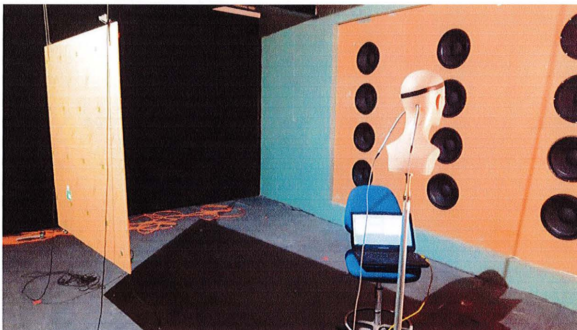
Figure 5: Manikin at RHS hotspot set at 0^\circ position (facing speaker baffle)
