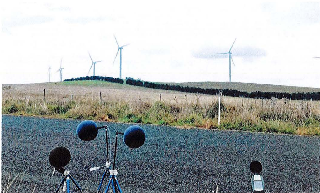
Figure 12: Multiple microphone setup
