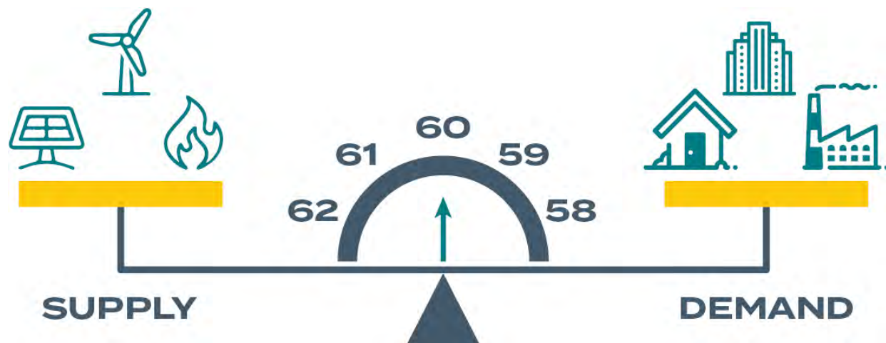
Figure 2. Maintaining Frequency: Energy Supply and Demand
